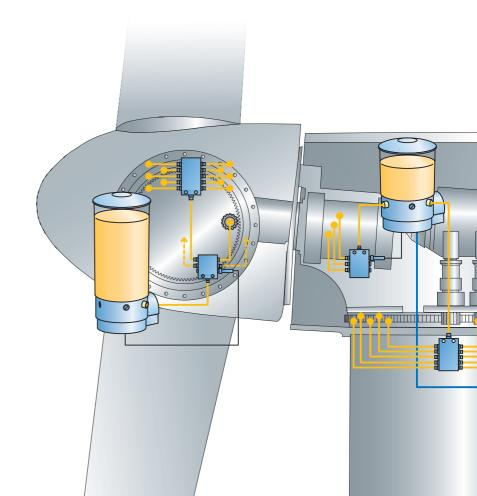
SKF offers lubrication system solutions tailored to every turbine application. Single-line and progressive automatic lubrication systems are available for pitch bearings, pitch open gears, main bearings, yaw bearings, yaw open gears and generators, while circulating oil systems are available for gearboxes. SKF also offers lubrication pinions for gear drives and suction elements that remove used grease from bearings.
