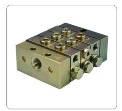
In this group, the feeder sections have two outlets on each side, one each on the side and one on top, but only one may be used. The second outlet must always be kept closed. These feeders are supplied with a built-in check valve.
