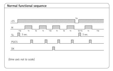
tp = interval time 30 = battery + / vehicle network = operating voltage + / after ignition "ON" 15 31 = operating voltage -= pushbutton / intermediate lubrication or pulse-counter input DK/MK PS/CS = pressure switch / cycle switch М = pump motor = indicator light SL Ζ = ignition lock = 5 A fuse
