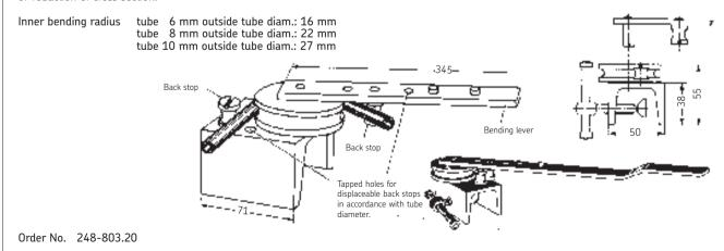
There is a special grooved disk available for the bending tube with 12 mm o.d, order No. 248-803.17
