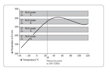
Penetration curve of a grease belonging to NLGI grade 2 as a function of temperature changes
