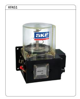
Pumps belonging to the KFA(S) series come with a maximum of 2 outlet ports for the connection of 2 independent lube circuits. A separate pump element is required for each outlet.
