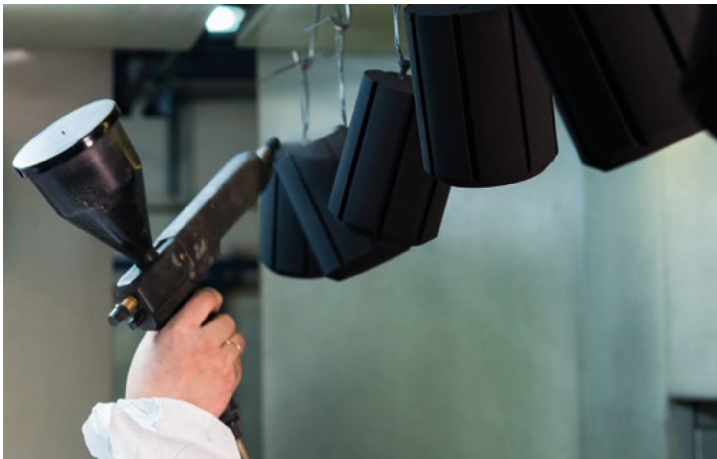
Powder coating of hanging components
