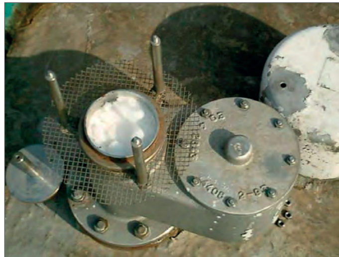
Clogging by crystallized acetic acid
