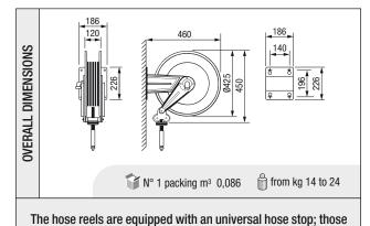
with hose are provided with a 0,6 m inlet connection hose.
