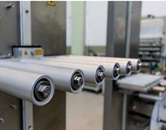
xiros® ball bearings in guide rollers Source: igus® GmbH
